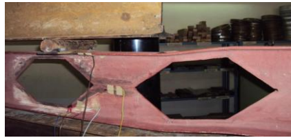
Fig. 1 Flexure Buckling of Castellated Beam
